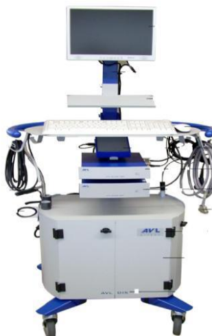
Fig 3: Emission Test Machine used in Bio Diesel Emission
