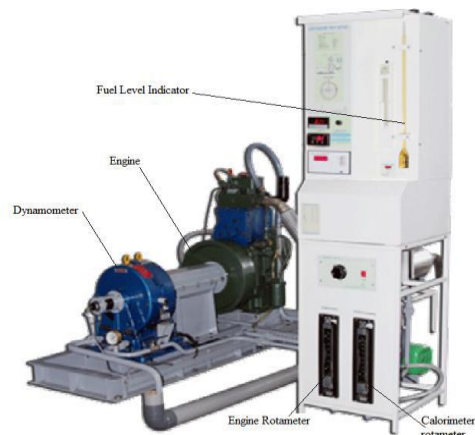
Fig 2: Single Cylinder Four Stroke Diesel Engine Kirloskar 1 Cylinder Use in Biodiesel Testing
